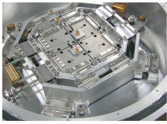
The FourStar detectors are four HAWAII-2RG 2048x2048 arrays manufactured by Teledyne Scientific and Imaging (formerly Rockwell Scientific) mounted in a 2x2 format. The arrays will be read out by the new application-specific integrated circuit (the "SIDECAR" ASIC) devices designed by Teledyne.
