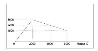
This disengages the slave axis at a specified master position. If the parameter is outside the master cycle, the stopping is instantaneous.
