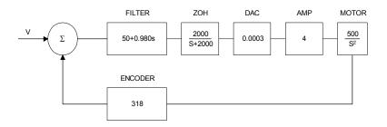
The open loop transfer function, A(s), is the product of all the elements in the loop.
