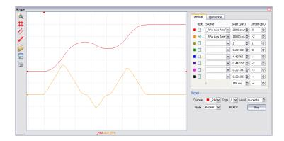
Note the controller treats the point where the velocity passes through zero as the end of one move, and the beginning of another move. IT is allowed, however it will introduce some time delay.
