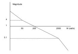
For the given example, the crossover frequency was computed numerically resulting in 200 rad/s.
