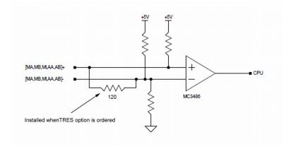
**Single-Ended Encoders:** Single-ended encoders will not operate correctly with the termination resistors installed. If a combination of differential encoder inputs with termination resistors and single ended encoders is required on the same controller, contact Galil directly.
