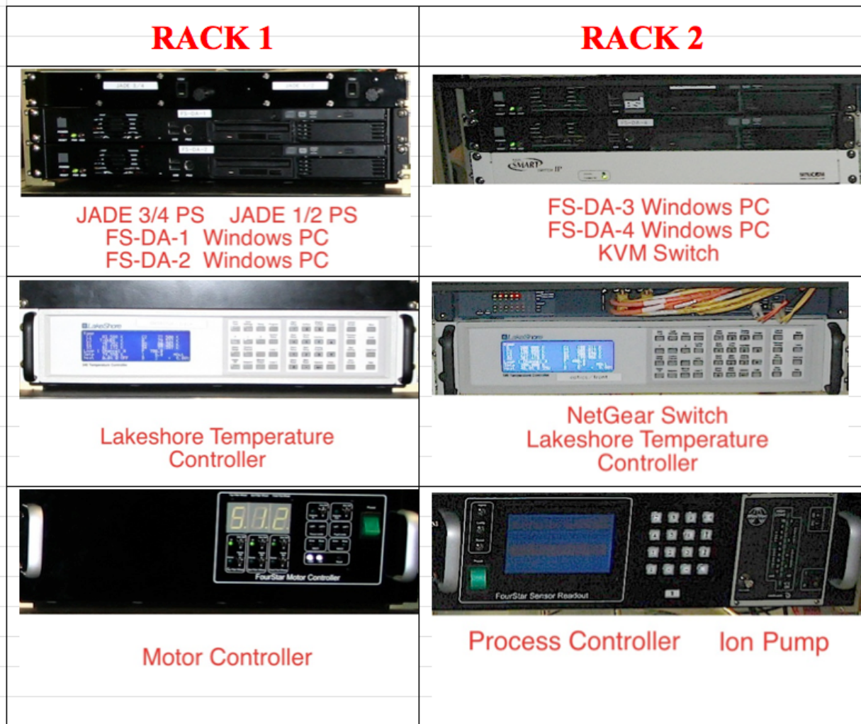
Figure 2. Electronics chassis in the 2 racks.
