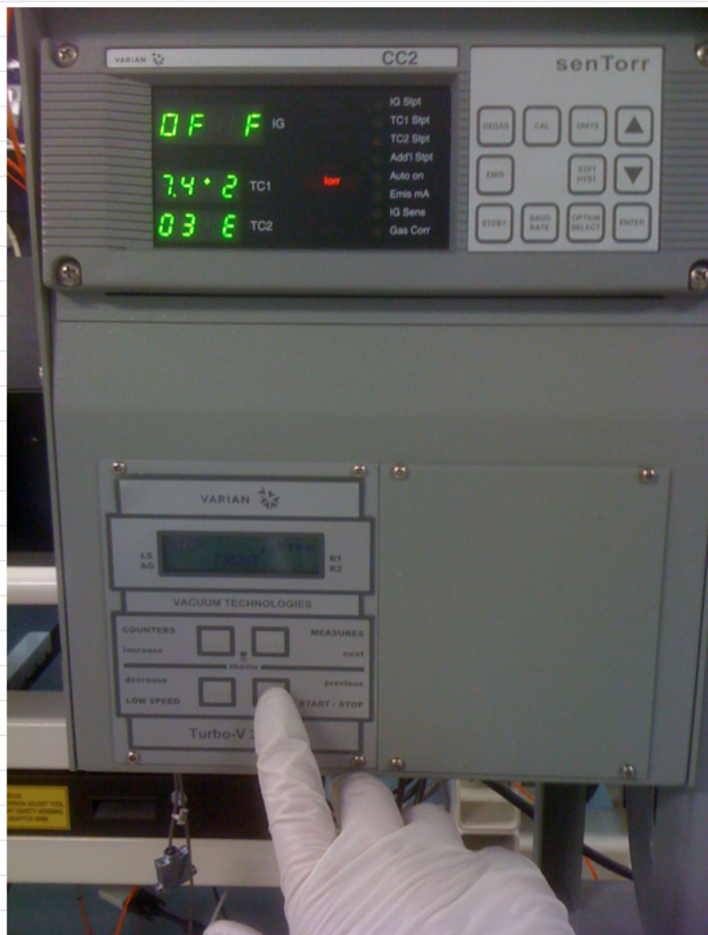
Figure 5. Turbo-pump control panel.
