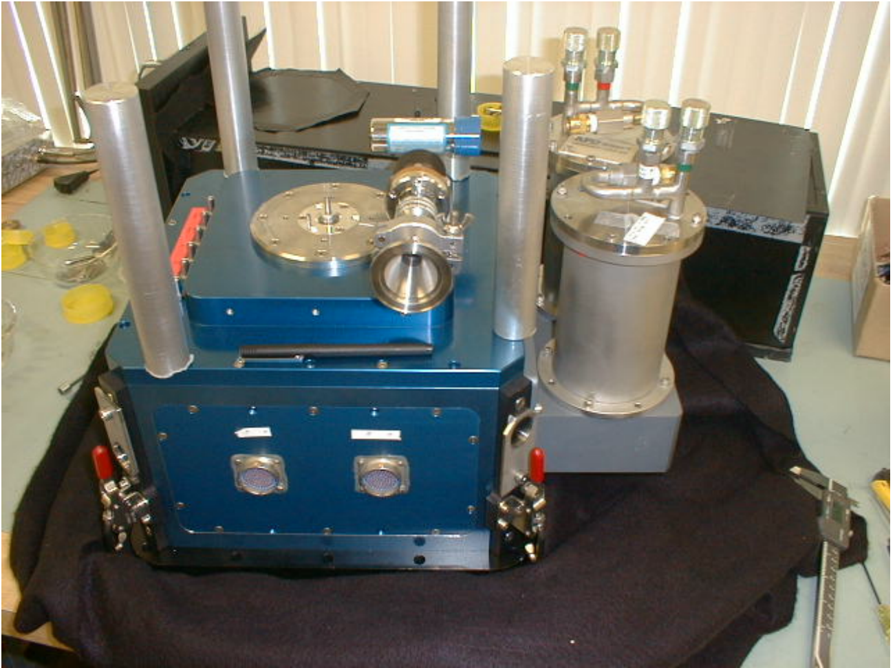
Figure 4. Dewar assembly showing dewar body, twin Cryotigers, and mounting latches. The four cylindrical legs are used only during assembly.
