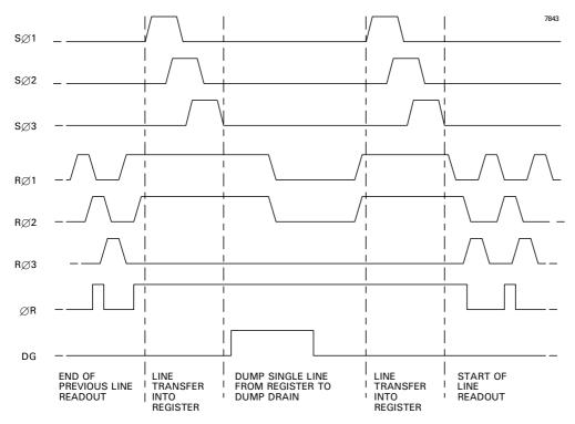
**DETAIL OF VERTICAL LINE TRANSFER (Multiple line dump)**
