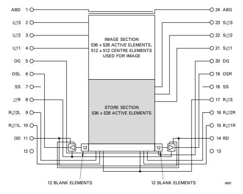
**Note** Pins 12 and 13 are not connected. For convenience, the CCD57-10 Compact Pack is pin compatible with the CCD47-10 sensors in the compact pack, except that OSL = pin 12, OSR = pin 13 and pins 6 and 19 are not connected in the CCD47-10.
