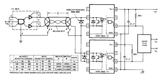
Figure c. Polarity Reversing, Split Phase.
