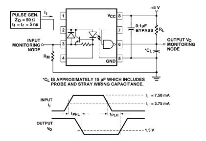
Figure 6. Test Circuit for  $t_{\mbox{\tiny PHL}}$  and  $t_{\mbox{\tiny PLH}}$
