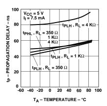
Figure 7. Typical Propagation Delay vs. Temperature.
