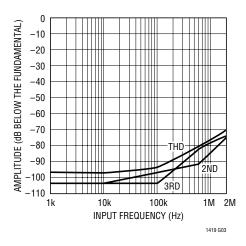
Figure 4. Distortion vs Input Frequency
