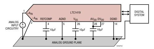
Figure 12. Power Supply Grounding Practice
