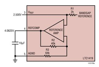
Figure 8a. LTC1419 Reference Circuit
