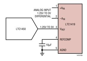
Figure 9. Driving V<sub>REF</sub> with a DAC
