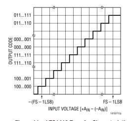
Figure 11a. LTC1419 Transfer Characteristics
