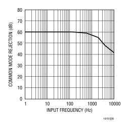
Figure 10a. CMRR vs Input Frequency
