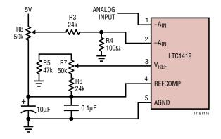
Figure 11b. Offset and Full-Scale Adjust Circuit
