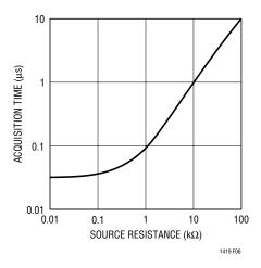
Figure 6. t<sub>ACQ</sub> vs Source Resistance
