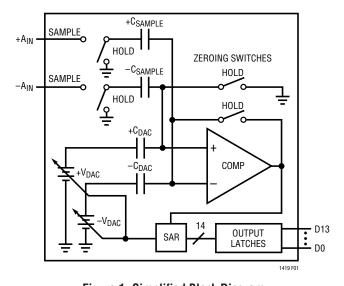
Figure 1. Simplified Block Diagram
