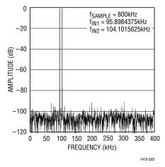
Figure 5. Intermodulation Distortion Plot
