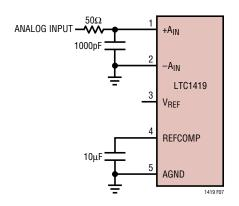
Figure 7. RC Input Filter
