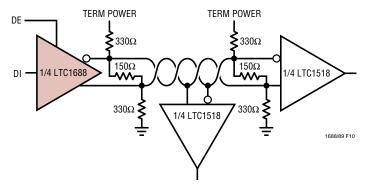
Figure 10. DC-Biased Termination (Recommended for SCSI Applications Only)
