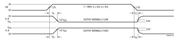
Figure 5. Driver Enable and Disable Times
