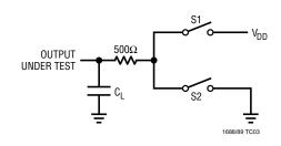
Figure 3. Driver Timing Test Load
