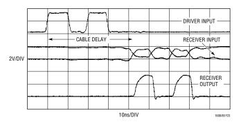
Figure 23. 25 Feet, 100Mbps, BRF2A Receiver
