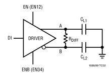
Figure 2. Driver Timing Test Circuit
