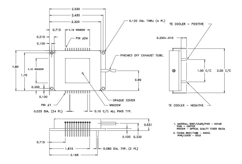
FIGURE 6 SIA003A package configuration
