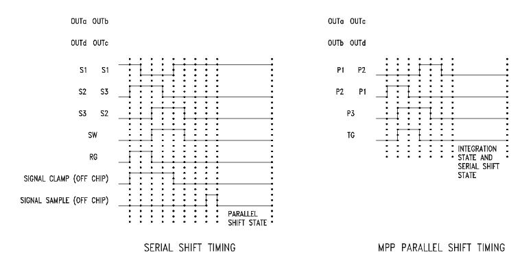
FIGURE 3 Serial and Parallel timing for all outputs
