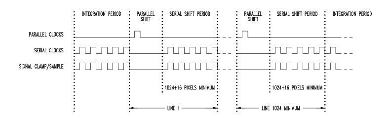
FIGURE 4 Typical full-frame readout
