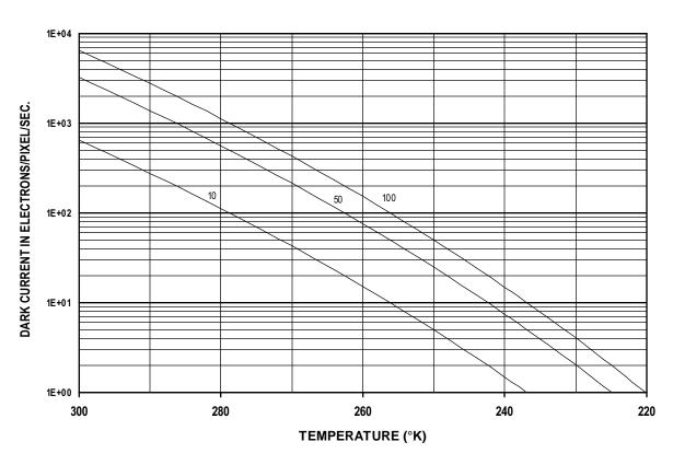
FIGURE 8 Effect of temperature on dark current. Parameter is pAmp/cm<sup>2</sup> at 293K
