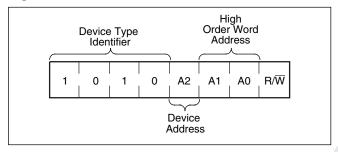
The next bit addresses a particular device. A system could have up to two X24C08 devices on the bus (see Figure 10). The two addresses are defined by the state of the A2 input.
