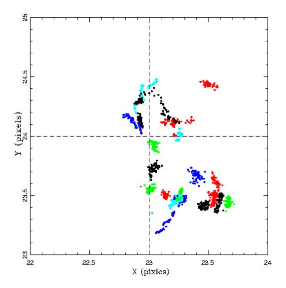
These are data from a two-night simulation of observing with the f/2 camera and the 300 l/mm grism. For each observation IMACS was slewed to a new position representing a random position in the southern sky, followed by 50 minutes of "tracking" at the proper speed. Open-loop flexure control was used. The grism was unlatched and relatched between exposures. The system shows excellent repeatability and sub-pixel drifts during exposures.
