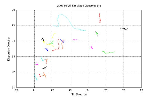
This is an equivalent test of the f/4 camera with the 1200 l/mm reflection grating. The brake that has been installed to steady the wheel while the latchup occurs has improved the repeatability, but there is still a quadrant of rotation when the image shifts by 3-4 pixels. In addition, there are some instances of significant wander during an exposure. Although this performance is acceptable for beginning observations, we will continue to investigate and refine the operation of this system.
