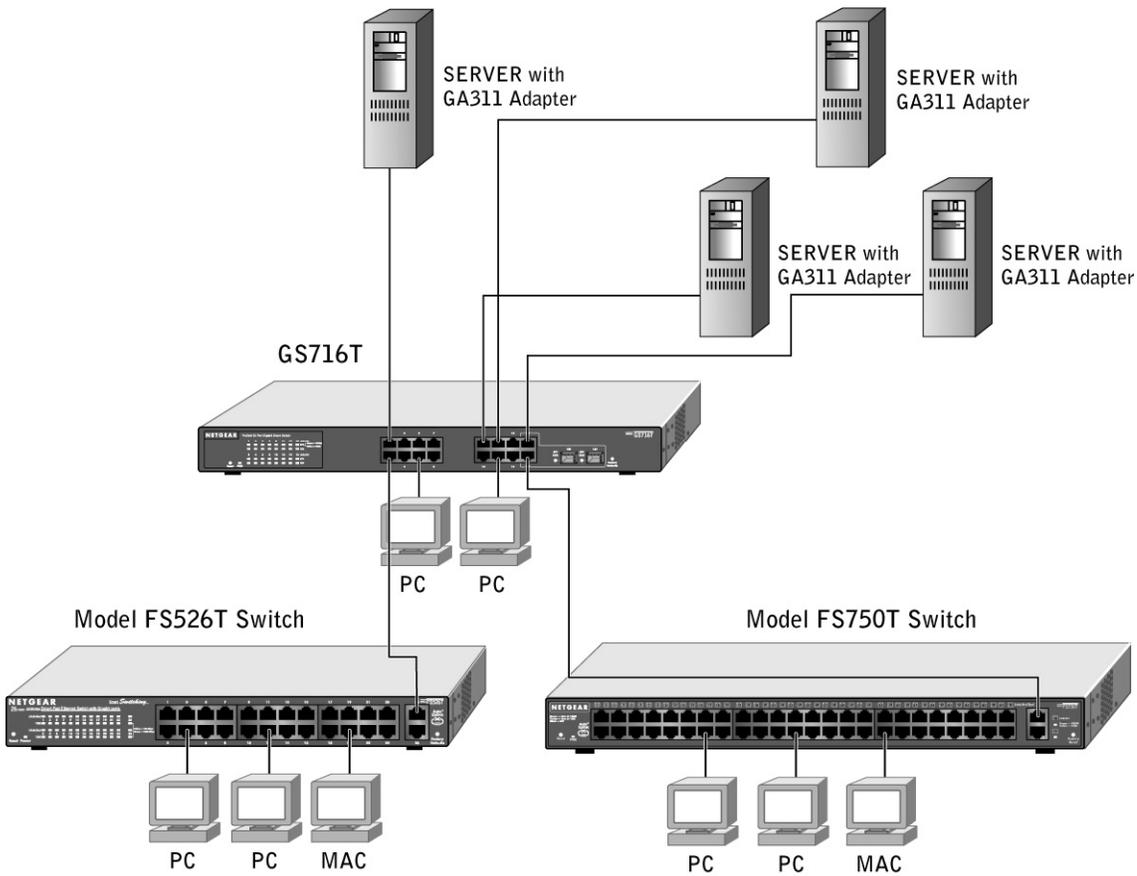
Figure 3-2. Example of Backbone Switching
