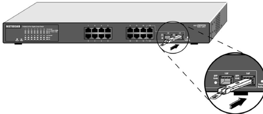
**Figure 4-3. Installing a SFP GBIC Module into GS716T**
