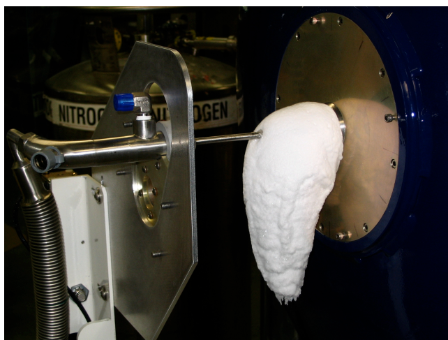
Figure 4.9 The autofill system with shroud dewar stinger in place. Note the ice build up near the fill tube.
